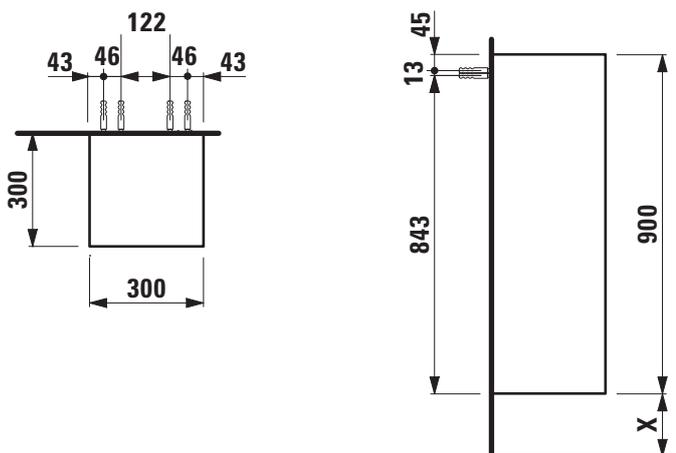
X = The exact height must be set during installation.
