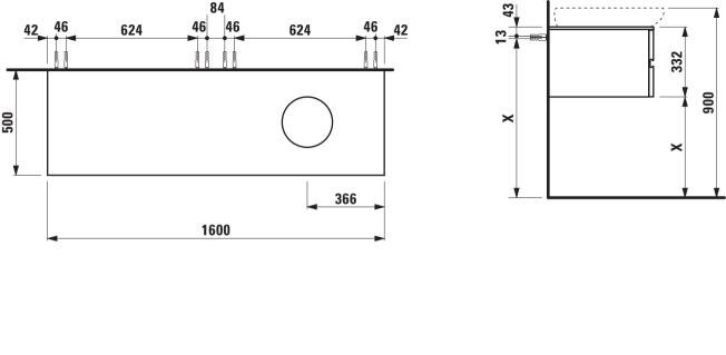
Only II Bagno Alessi One 81897.3 with shelf at left side X = The exact hight must be set during installation.
