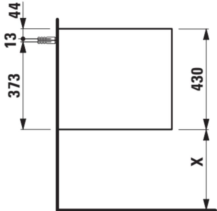
X = The exact height must be set during installation.
