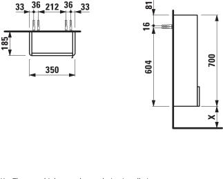
X = The exact hight must be set during installation.
