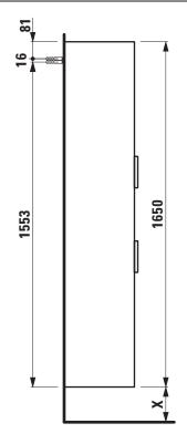
X = The exact hight must be set during installation.
