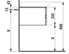
Only II Bagno Alessi One  $\epsilon$ 1897.3 with shelf at left side X = The exact hight must be set during installation.
