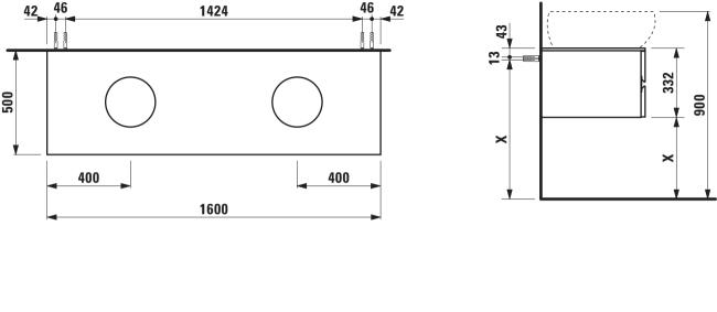
X = The exact hight must be set during installation.
