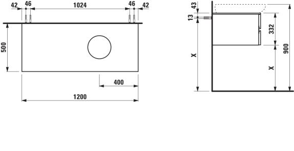
X = The exact hight must be set during installation.
