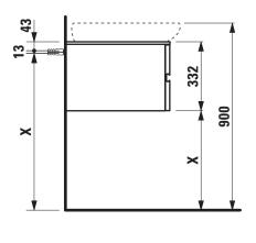
Only II Bagno Alessi One &1897.3 with shelf at left side X = The exact hight must be set during installation.
